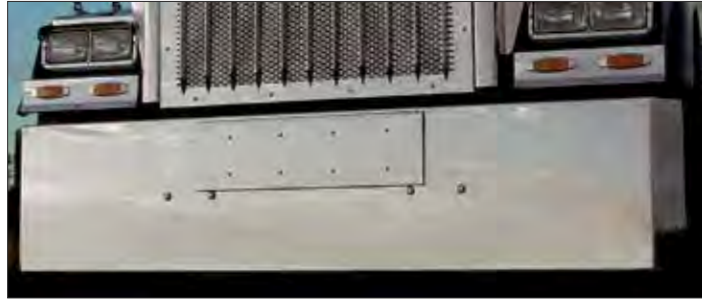
Standard Mount Blank Face Bumper with Mitered Ends, and Hinged Plate Hanger.
