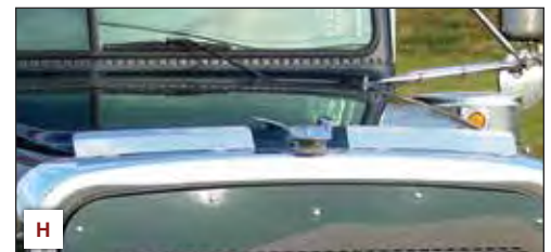
Triple Diamond Punched Grille Insert shown on Peterbilt Truck
